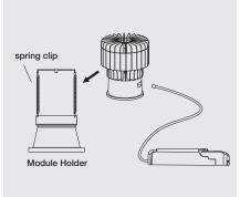
3. Attach module to module holder with spring clip and connect module to driver.
